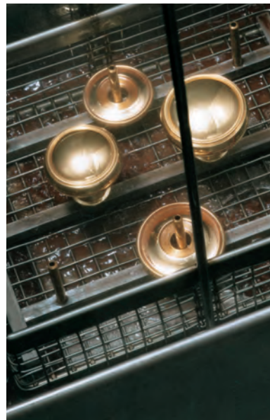
Hardware lowered into ultrasonic cleaner to remove any residual compounds left from the buffing and polishing process.
