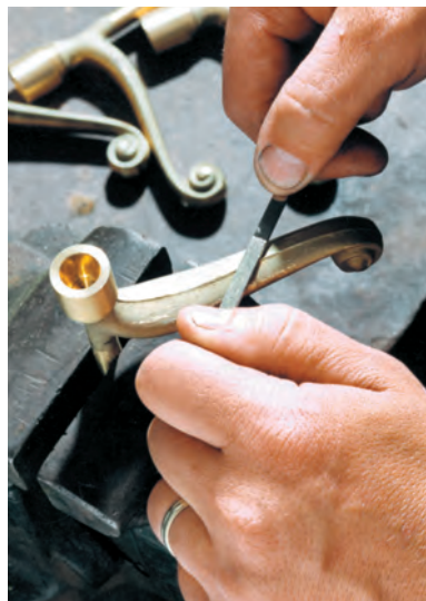
A craftsman files the parting line of a lever.
